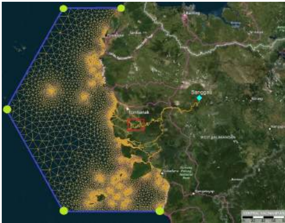
Figure 19: Domain extent and boundary conditions of the Delft3D-FM® numerical model. Red box below Pontianak outlines the junctions of interest. Blue polyline shows the semi-hexagonal edge at the sea. Green points at the corners of the polyline indicate locations of the downstream B.C. Cyan diamond at Sanggau indicates the location of the upstream B.C.
