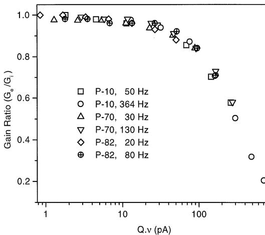
Fig. 7. Comparison of the variation of the relative gains ( $G_e/G_i$ ) for three different argon/methane mixtures as a function of the current produced in the external cathode section of detector B, by the ionizing radiation.
