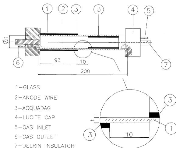
Fig. 1. Schematic drawing of the resistive cathode proportional counter.
