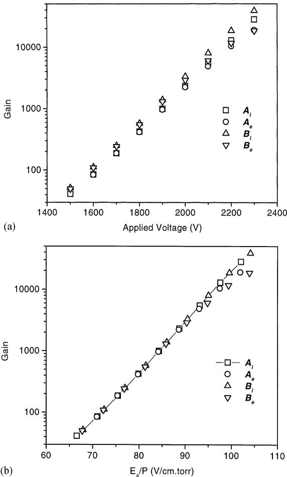
Fig. 2. Measured gains in the P-10 mixture, for detectors A and B (for both internal and external cathode sections), as a function of: (a) the applied voltage; (b) the reduced electric field at the anode computed for the internal cathode detectors.
