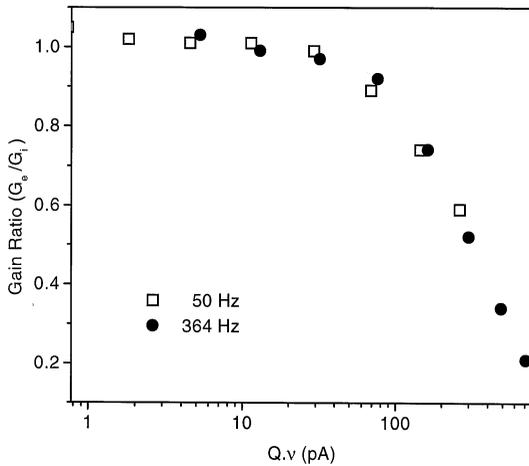
Fig. 6. Ratios  $G_e/G_i$  for the P-10 mixture as a function of the current produced in the external cathode section of detector B (equipped with a  $50 \mu\text{m}$   $\phi$  stainless steel wire) by the ionizing radiation, for two counting rates.
