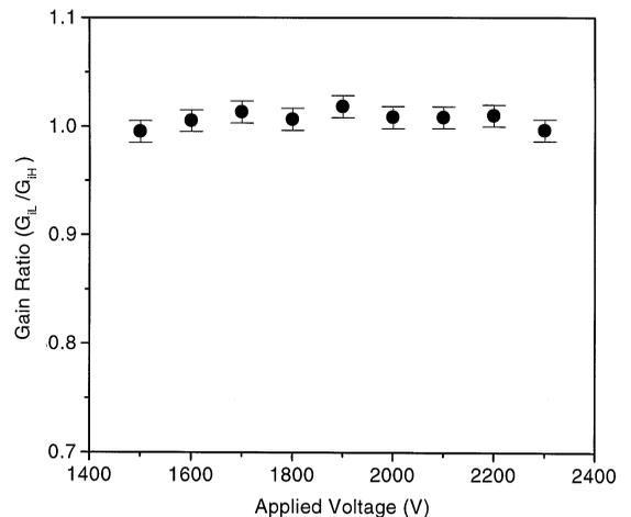
Fig. 3. Ratio ( $G_{iL}/G_{iH}$ ) between the gains measured in the P-10 mixture for detector  $A_i$  (internal cathode) at the lowest and the highest counting rates, 70 and 510 Hz, respectively, as a function of the applied voltage.
