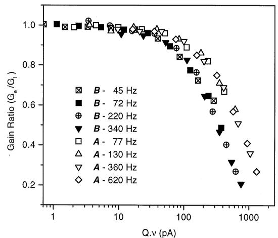
Fig. 5. Comparison of the variation of the relative gains ( $G_e/G_i$ ) shown in Fig. 4a and 4b, as a function of the current produced in the external cathode detector by the ionizing radiation.
