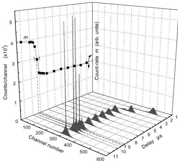
Fig. 5. Pulse-height spectra recorded by the MCA, as a function of the delay of the electronic pulses. Count-rate (■) in arbitrary units. Pulse amplitude is 3.3 V.
