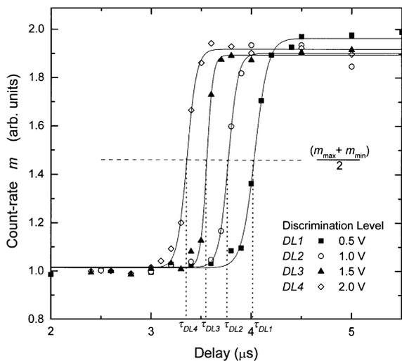
Fig. 3. Dead times for several discriminator levels (DL) of the pulse discriminator, with the GPSC → PD–EC counting system, with a pulse amplitude of 3.5 V.
