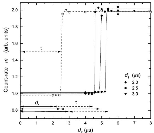
Fig. 6. Dead times (○) for a PD–EC counting system with a pulse amplitude of 2.8 V. Behavior of this counting system, see text, with  $d_1 = 2.0 \mu\text{s}$  (◆),  $d_1 = 2.5 \mu\text{s}$  (●) and  $d_1 = 3.0 \mu\text{s}$  (▼).
