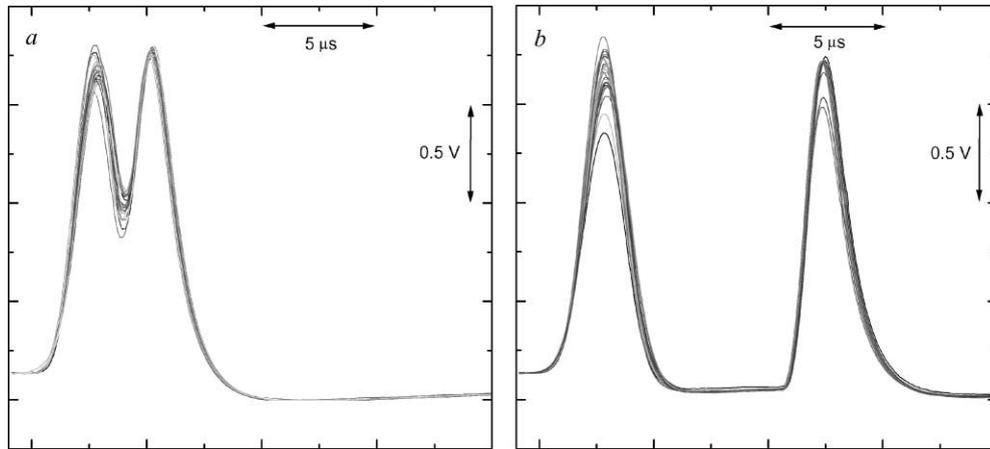
Fig. 2. Digitized form of the pulses (sampling rate of 1.25 MHz) of a typical sequence. The first set of pulses in each figure corresponds to 5.9 keV X-ray events in a gas proportional scintillation counter filled with Xe–10% Ar. The pulses in the second set are generated electronically by the first pulses after a delay of 4 μs (a) or 10.5 μs (b).
