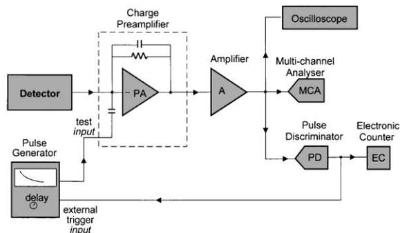
Fig. 1. Experimental setup for the measurement of the counting system effective dead time.
