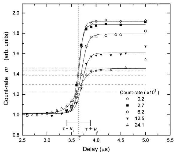
Fig. 4. Dead times for several detector counting-rates, with the GPSC (Xe-10% Ar)  $\rightarrow$  PD-EC counting system, with a pulse amplitude of 3.3 V.
