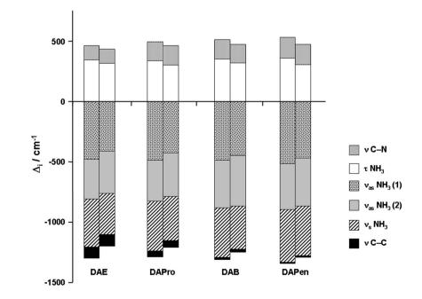
of the  $\Delta_i$ -values ( $\omega_i$ (amine-HCl)- $\omega_i$ (amine-H)) for some selected vibrational modes, as a function of diamine and theory level. In each set, left and right columns refer to the mPW1PW/6-31G\* and  $\omega$ B97XD/6-311++ G(2d,2p) results, respectively
