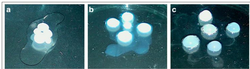
Figure 14. CMC-Cht particles a) without any additive, with b) SL and c) SC.
