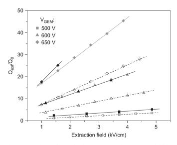
Fig. 4. Dependence of amplification  $Q_{\rm ext}/Q_0$  on the extraction field for several values of  $V_{\rm GEM}$  at  $\rho = 6.1 \times 10^{19} \, {\rm cm^{-3}}$ . Gray symbols—saturated gas, black symbols—two phase mode, open symbols—gas at  $-90 \,^{\circ}{\rm C}$ .
