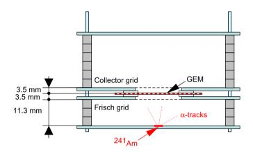
Fig. 1. The ionisation chamber used in the measurements (5.49 MeV  $\alpha$ -particles, emitted by <sup>241</sup>Am, have range of 11 mm in Xe gas with density  $4.9 \times 10^{19} \text{ cm}^{-3}$ ).
