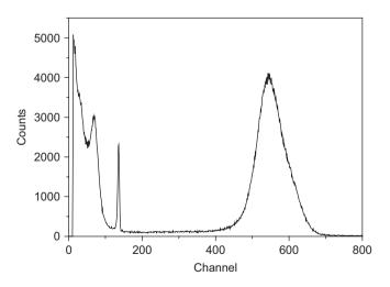
Fig. 5. Pulse-height spectrum obtained in the two-phase mode.  $V_{\text{GEM}} = 625 \text{ V}, \ Q_{\text{ext}}/Q_0 = 15$ . Narrow peak at channel 130 is due to calibration pulses.
