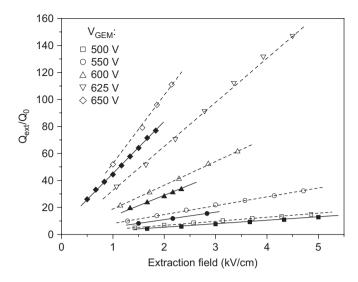
Fig. 3. Dependence of amplification  $Q_{\text{ext}}/Q_0$  in xenon gas on the extraction field for several values of  $V_{\text{GEM}}$ . Solid and open symbols correspond to 25 °C and -90 °C, respectively. Gas density is  $4.9 \times 10^{19} \text{ cm}^{-3}$ .
