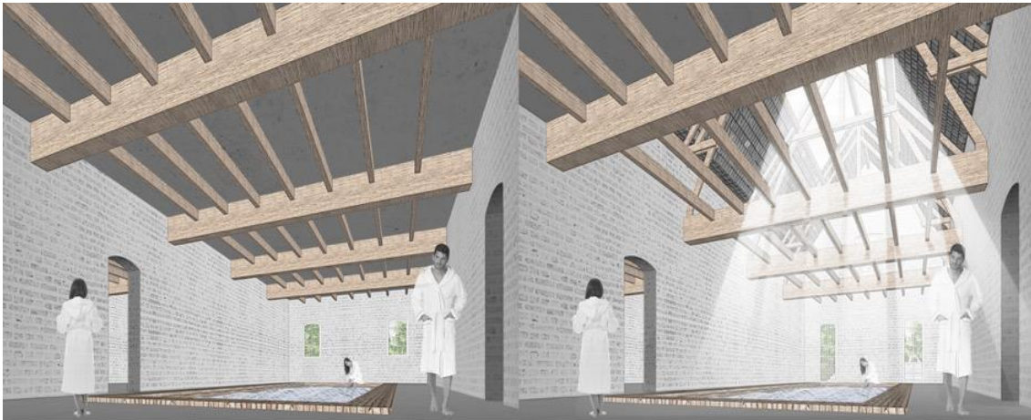
Figure 3 - Different scenarios of a wellness: one without additional openings (see on the left) and one with additional openings (see on the right).
