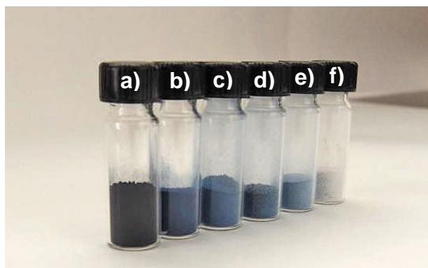
Figure 7.1 – Picture of the obtained LDH materials: a) IC-LDH, b) IC(3.9%)/HS-LDH, c) IC(2.2%)/HS-LDH, d) IC(1.1%)/HS-LDH, e) IC(0.6%)/HS-LDH and f) HS-LDH.
