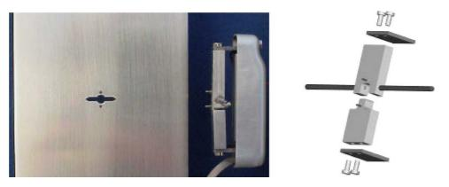
Fig. 2. Pin microgauge and corresponding position in the specimen.
