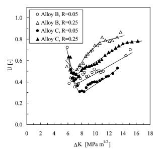
Fig. 6. Influence of the stress ratio on the crack closure level for alloys  $B \mbox{ and } C.$
