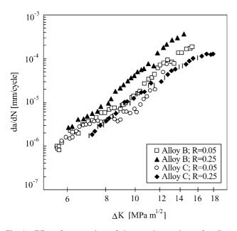
Fig. 4. Effect of stress ratio on fatigue crack growth rate for alloys B and C.
