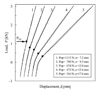
Fig. 3. Typical load-displacement records for alloy A.
