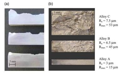
Fig. 8. Images of specimens: (a) typical crack paths; (b) fatigued fracture surfaces.
