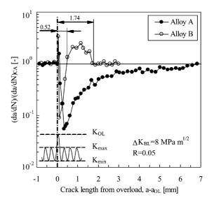
Fig. 10. Transient crack growth rate following a single tensile overload.
