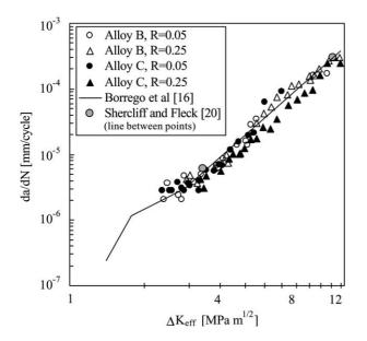
Fig. 9. Fatigue crack growth rate versus  $\Delta K_{\rm eff}$  for AlMgSi1-T6 alloys.
