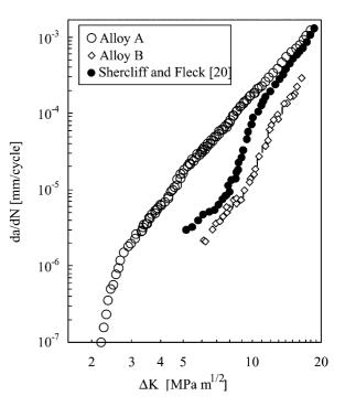
Fig. 5. Fatigue crack growth rates for different AlMgSi1-T6 aluminium alloys at R = 0.05.
