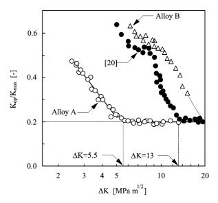
Fig. 7. Crack closure data for AlMgSi1-T6 Alloys. R = 0.05.
