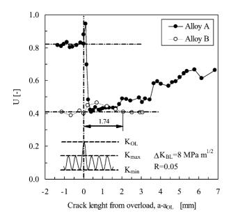
Fig. 11. Crack closure response following a single tensile overload.
