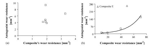
Fig. 7. Wear resistance of the composites vs. wear resistance of the antagonist in the reciprocating test with: (a) abrasive slurry and (b) saliva.
