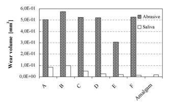
Fig. 4. Comparison of wear volumes of the restorative materials for the reciprocating test with: abrasive slurry and artificial saliva.
