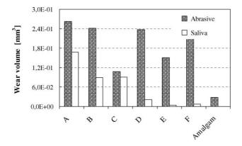
Fig. 5. Wear volumes of the antagonist body for the reciprocating test with: abrasive slurry and artificial saliva.
