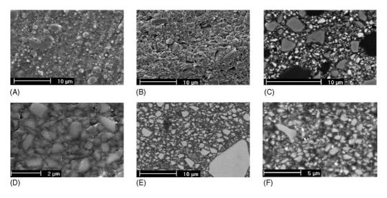
Fig. 1. Morphology of the composite materials observed by SEM.
