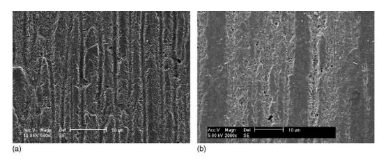
Fig. 8. Morphology of the composite specimens in the reciprocating test with: (a) abrasive (composite E) and (b) saliva (composite B).
