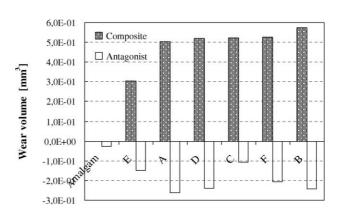
Fig. 3. Wear volumes of the restorative materials and the antagonist body, for the reciprocating test with abrasive slurry.
