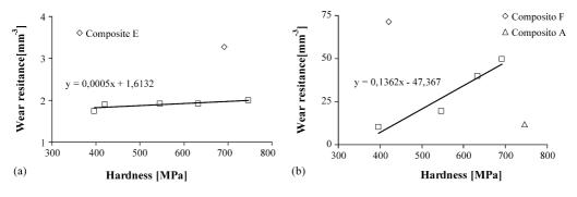
Fig. 6. Hardness vs. the wear resistance of the composites for the reciprocating test with: (a) abrasive slurry and (b) saliva.
