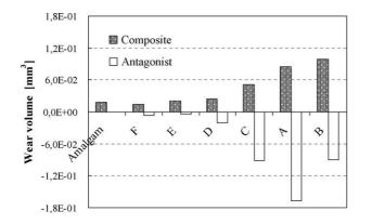
Fig. 2. Wear volumes of the restorative materials and the antagonist body, for the reciprocating test with artificial saliva.
