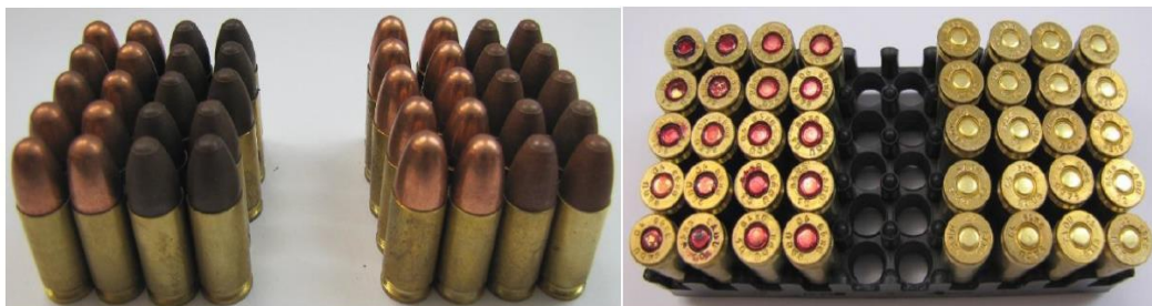
Figure 3.9. The four 9 mm small calibre ammunition, with combination of two different projectiles and primers (Rotariu et al. , 2015).
