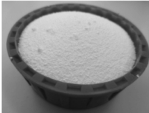
Figure 1: Photographic view of the microencapsulated PCM used to fill up the TES units - Micronal® DS 5001 X
