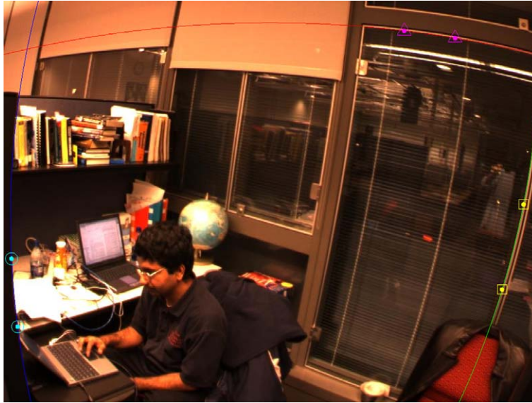
Fig. 5. Estimation of the distorted projection of a line from two image points selected by hand. The image size is 768 \times 1024 and the radial distortion causes a displacement of 273.55 pixels at the image corner. The conic curve \Omega'' , corresponding to the projection of a line, is estimated from two image points knowing that \Omega'' must go through the circular points and satisfies \mathbf{M}''^T \Omega'' \mathbf{N}'' = 0 (Eq. (27)).
