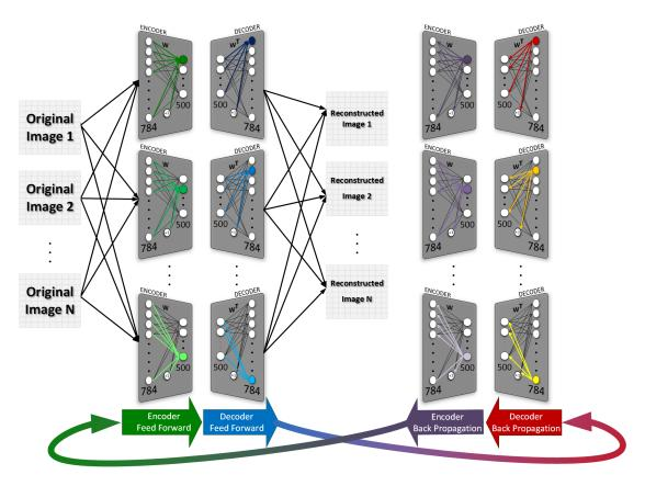
Figure A.1: Detailed autoencoder flow diagram
