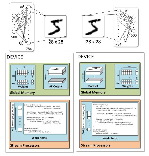
Figure 4.3: Back propagation work-items for the output layer (decoder)
