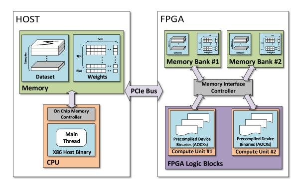
Figure 4.5: Architecture of the FPGA running the OpenCL kernels on two CUs
