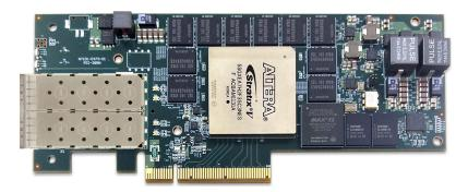
Figure 5.4: The Altera Stratix V D5 from Nallantech [9]
