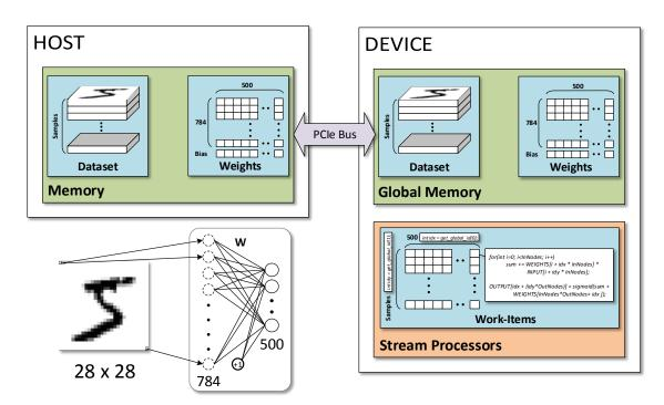
Figure 4.2: Feed forward work-items spread across two dimensions
