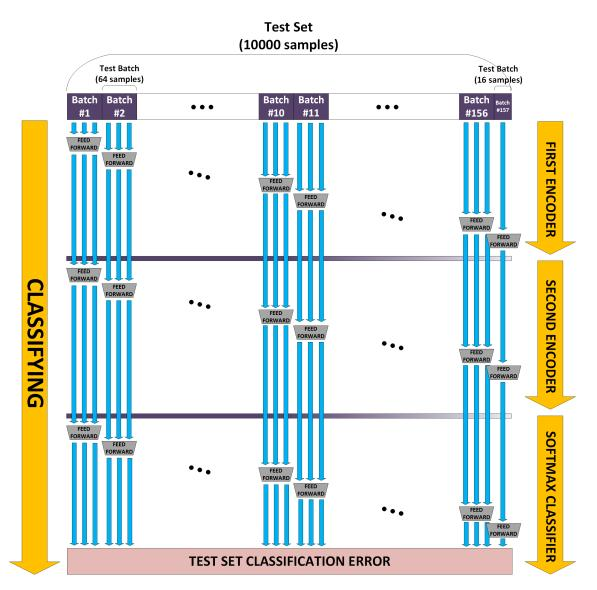
Figure A.7: Test set classification flow diagram
