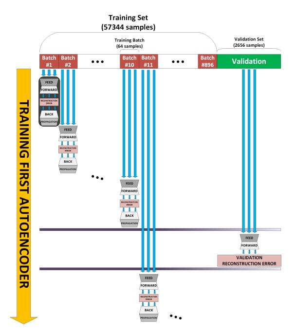
Figure A.3: First autoencoder training flow diagram. The detailed execution flow of the autoencoder in the shadowed area below Batch #1 is explained in Fig. A.1
