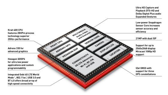
Figure 3.5: The Qualcomm Adreno 330 GPU in the Snapdragon 800 SoC [4]
