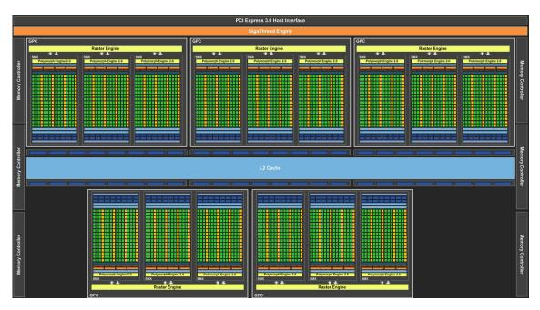
Figure 3.3: The Nvidia GTX Titan (GK110) GPU block diagram [3]
