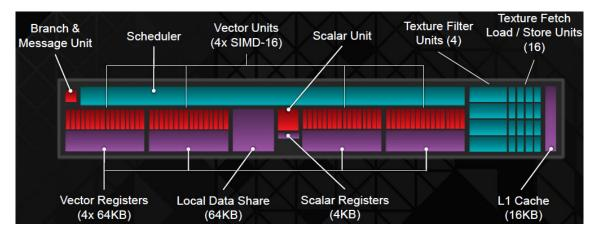
Figure 3.2: A detailed view of the GCN Architecture Compute Unit in the AMD R9 290X (Hawaii) [2]
