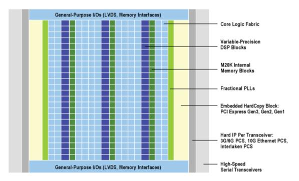
Figure 3.6: Stratix V FPGA architecture and features [5]
