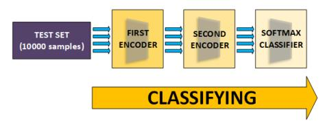
Figure A.6: Test set classification flow diagram. The classification flow is explained in more detail in Fig. A.7
