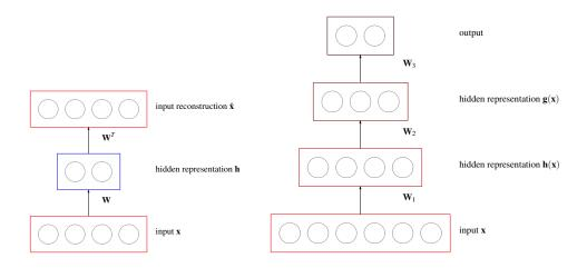
Figure 2.6: Example of an autoencoder (left) and of a stacked autoencoder (right).
