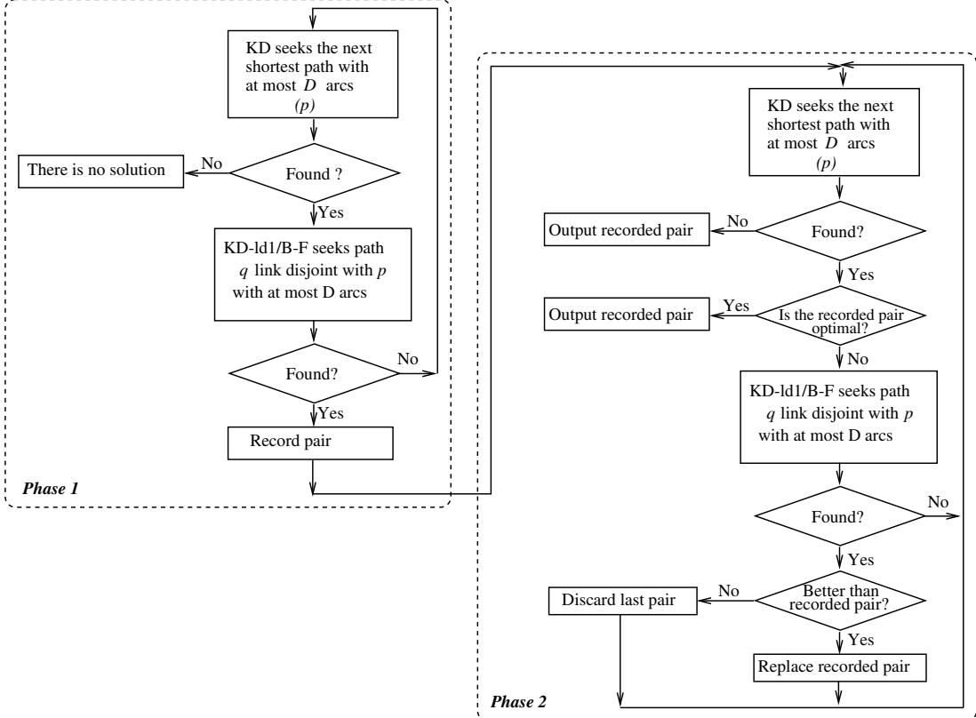
Fig. 1. Flowchart of proposed variants of the algorithm (RLDPC and RLDPC-BF).
