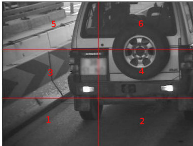
Figure 6.2: Image showing the different sections of the image used to train the different classifiers.
