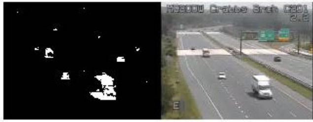
Figure 3.8: Background subtraction mask.
