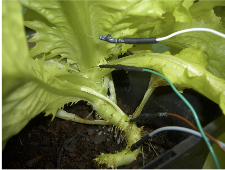
Figure 4.4: Electrode placement in lettuce, from bottom up: reference, root, base of the leaf and leaf.
