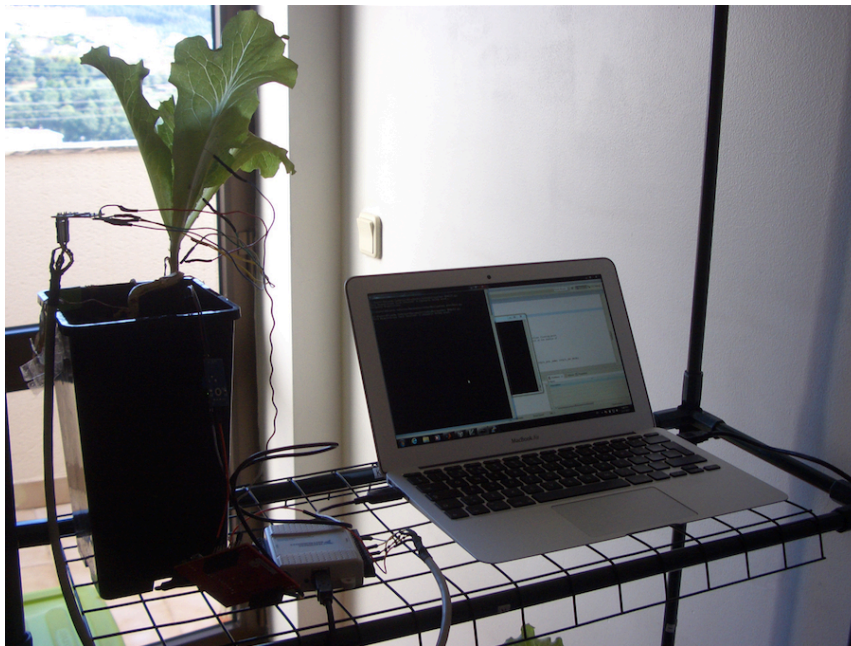
Figure 3.3: Example set-up for the tests on lettuce using Amplifier Circuit 1 and NI USB-6009.
