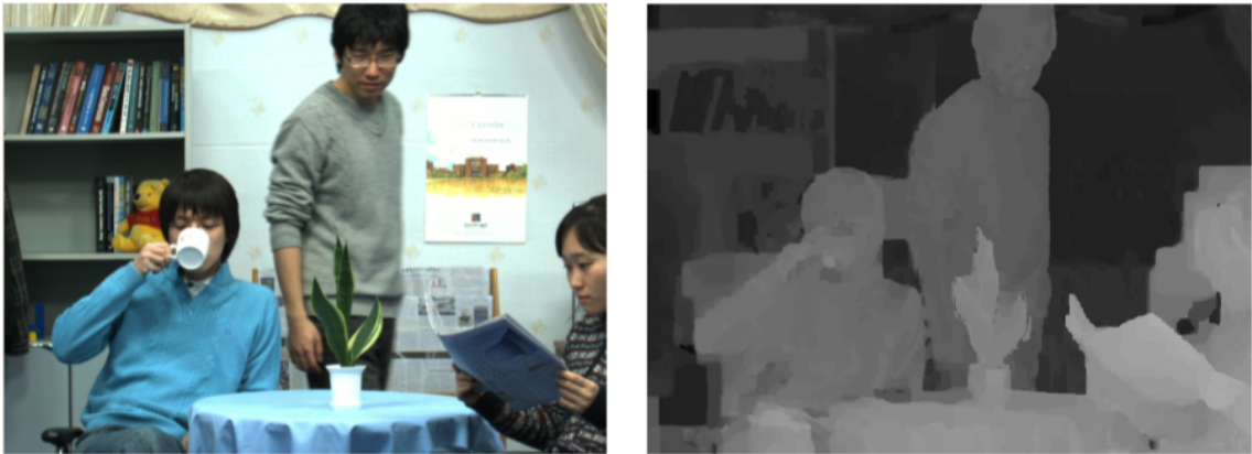
Figure 1.2: Example of a frame extracted from a 3D video in the texture-plus-depth format. The texture frame (left) has a correspondent per-pixel depth frame with depth information in the form of a depth map (right).
