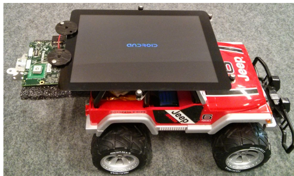
Figure 5.1: Prototype with SABRE SD platform on the RC car.
