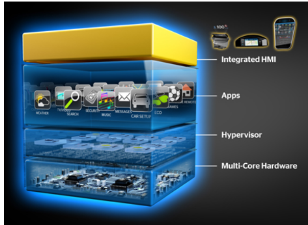
Figure 2.8: Integration via multi-core-hardware and Hypervisor [22].
