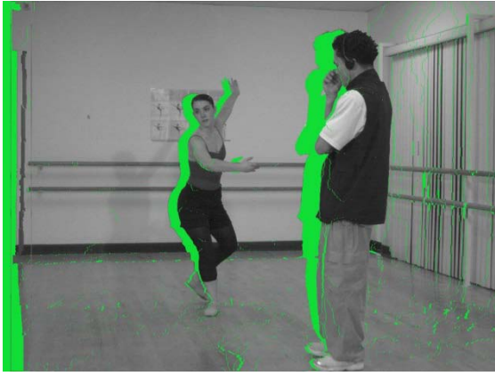
Figure 2.7 – Luminance 1 of the left and right synthesized views of the Ballet's 1 st frame, without hole-filling (the green color serves here only to highlight no-filled deoccluded regions, or holes).
