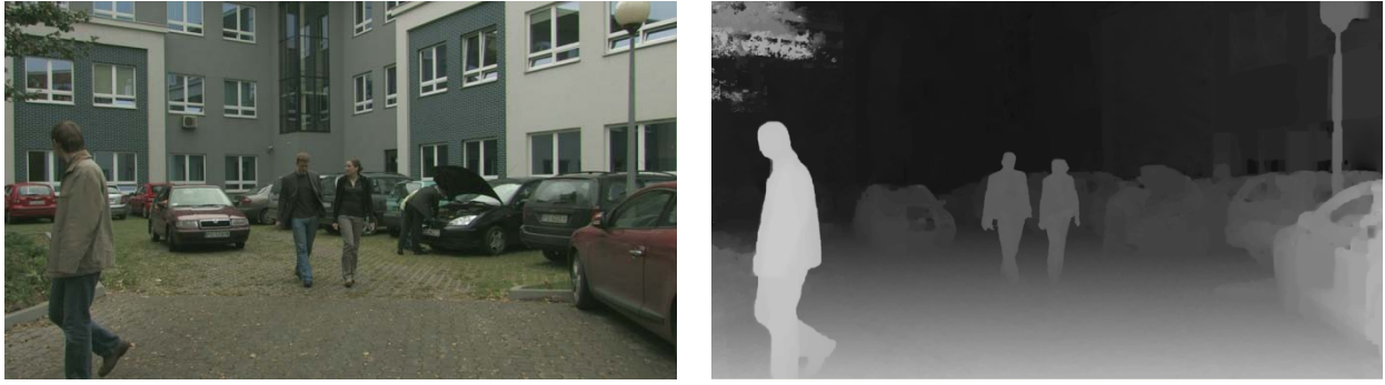
Figure 1.2 – Example of a frame extracted from a 3D video in texture-plus-depth format, which is the scope of this thesis. It consists of the texture frame (left) and the per-pixel depth information in the form of a depth map (right).
