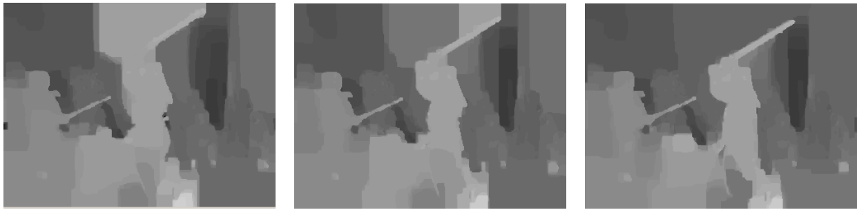
Figure 2.4 – Three consecutive depth frames from Kendo, to exemplify temporal inconsistencies from estimation.
