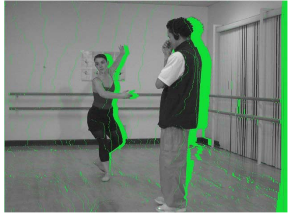
Figure 2.7 – Luminance 1 of the left and right synthesized views of the Ballet's 1 st frame, without hole-filling (the green color serves here only to highlight no-filled deoccluded regions, or holes).
