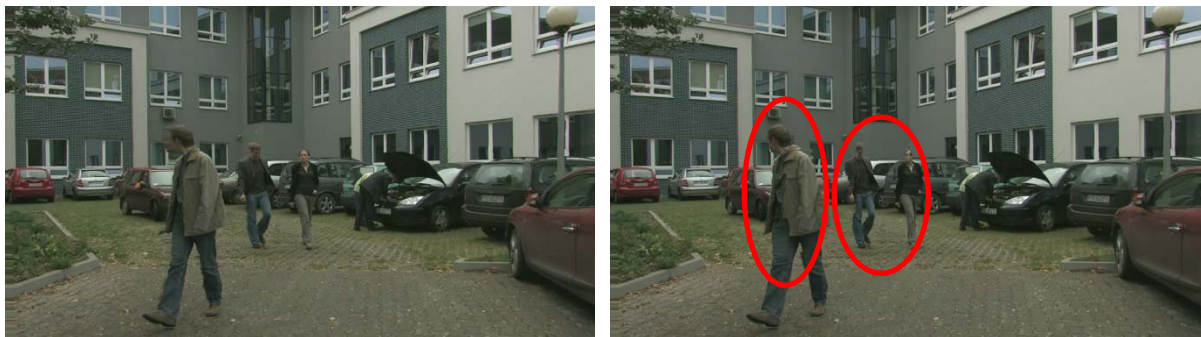
Figure 3.3 – Reference (left) and distorted (right) 120 th frame of a synthesized view of Poznan CarPark, extracted from a simulation with 20% PLR corrupted depth map. Red ellipses are only to point the most distorted zones. PSNR = 30.54 dB , SSIM = 0.938 (luminance component).
