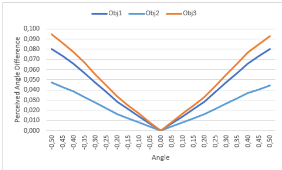
Figure 4.9: X axis rotation: Difference between the angle as seen by the real and corrected camera for each object (in degrees)
