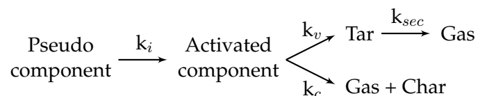
Figure 3.6: Miller-Bellan biomass pyrolysis scheme (1997) [40].
