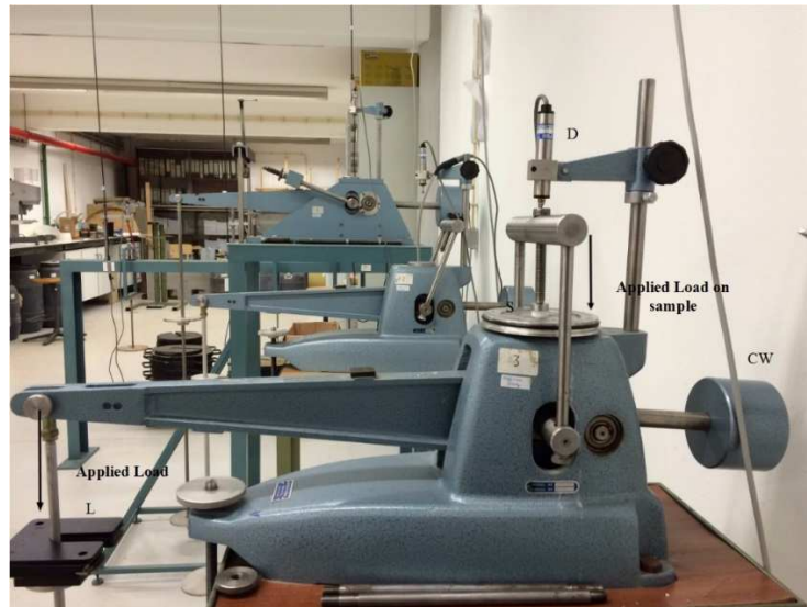
Figure 6. Employed oedometer for mechanical characterization of the produced biomaterials. D -deformation transducer; S – sample; CW – counterweight; L – applied load.
