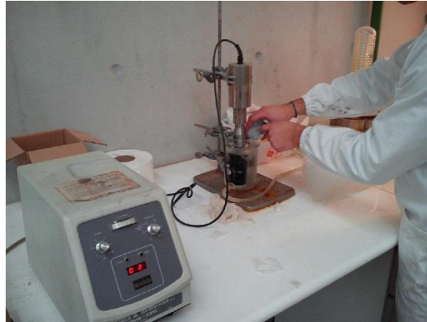
Figure 15 - Apparatus used during the application of ultrasounds to the suspension.
