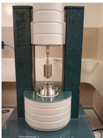
Figure 12 - Controlled stress reometer of Haake, model RS1.
