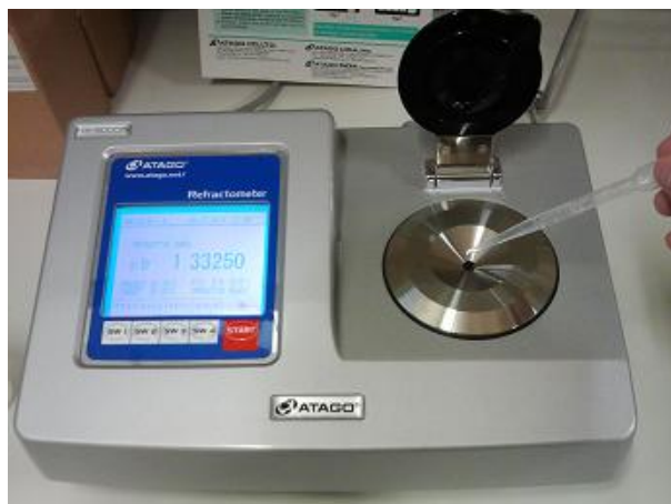
Figure 11 - Refractometer RX-5000D by Atago.
