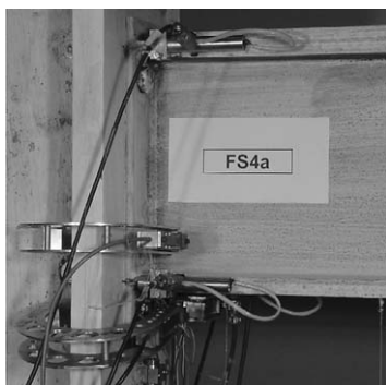
Fig. 6. MBs 1, 3 and LVDTs 6, 9 (illustration with specimen FS4a).
