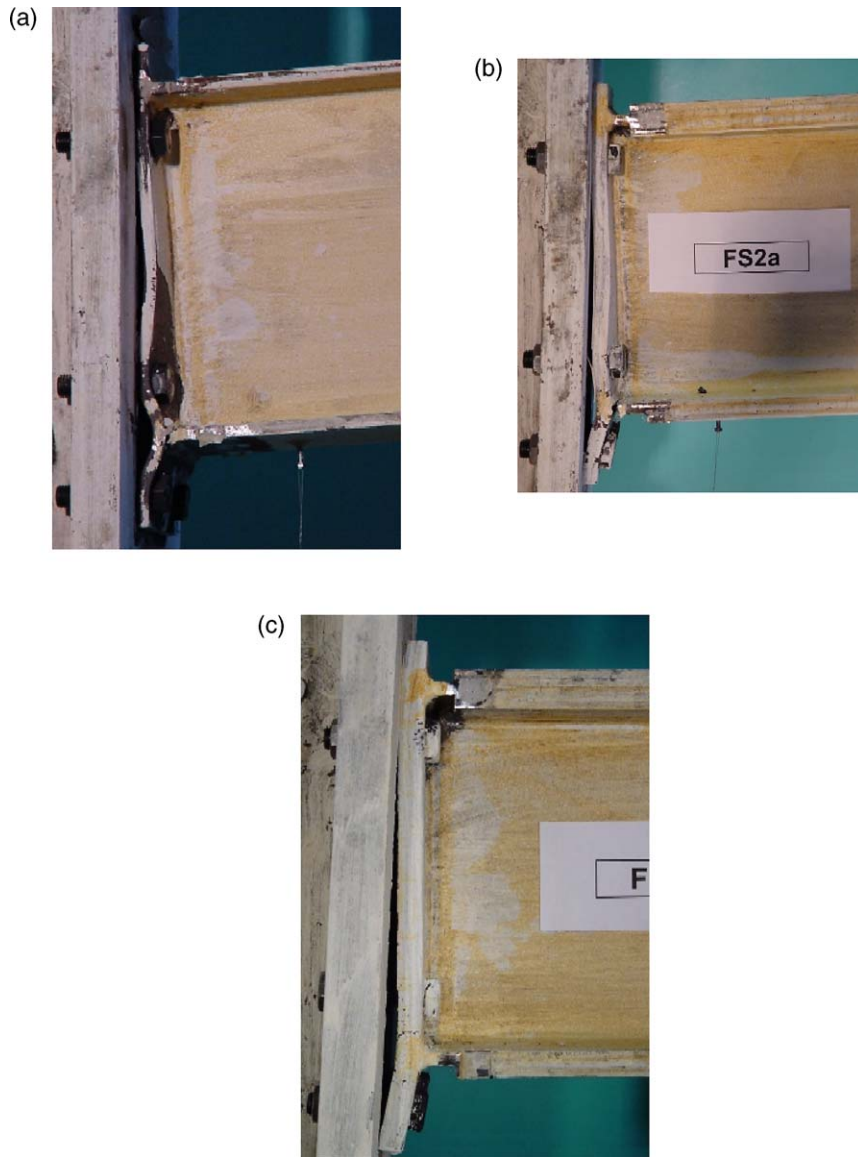
Fig. 19. Comparison of the end plate deformations at failure conditions for test series FS1-3. (a) Specimen FS1a. (b) Specimen FS2a. (c) Specimen FS3b.
