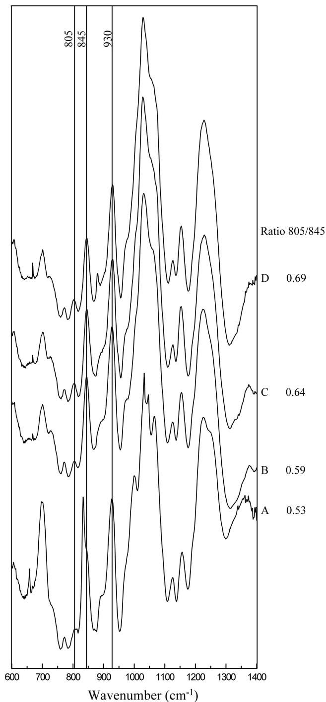
Fig. 1. FTIR spectra of alkali treated carrageenan: (A) *C. crispus* (non-fertile thalli), (B) *C. crispus* (female gametophytes), (C) *M. stellatus* (gametophytes), (D) *G. pistillata* (female gametophytes).
