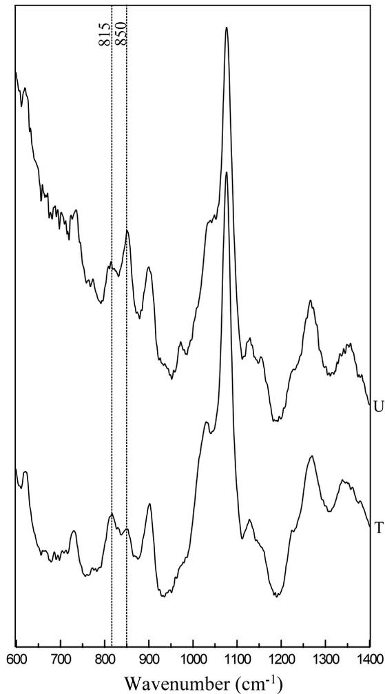
Fig. 7. FT-Raman spectra of alkali treated carrageenan: (T) *C. acicularis* (tetrasporophytes), (U) *C. teedei* var. *lusitanicus* (tetrasporophytes).
