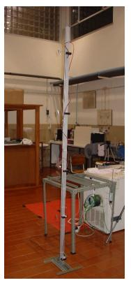
Figure 2.3. Thermistor vertical bar.
