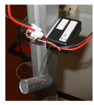
Figure 2.4. Thermistor with aluminium foil protection.
