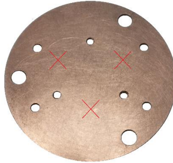
Figure 5.1. Cooper target and reference points of measurement of the thickness (represented as a cross).
