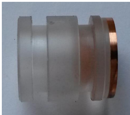
Figure 4.6. High velocity sabot.
