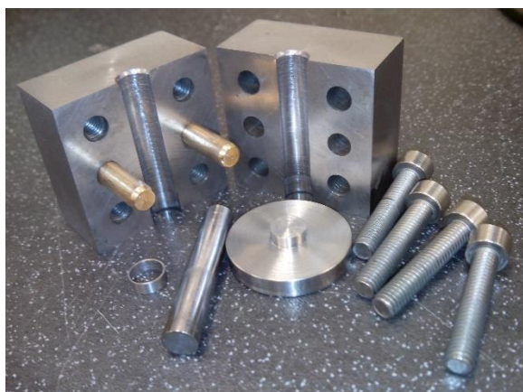
Figure 3.3. Isostatic compressing dye and ring.
