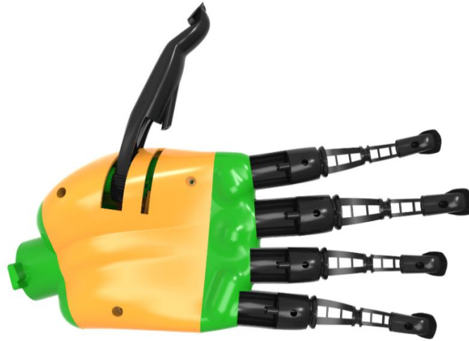
Figure 5.1 – 3D model of the robotic hand. It is possible to see the internal structures of the fingers (black), the main structure of the hand (green) and the palm cover (orange).
