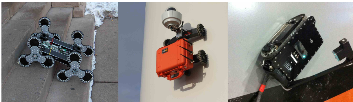
Figure 6: Wheel based climbing robots, from left to right: Wheg, Wheel and Caterpillar base Robots.
