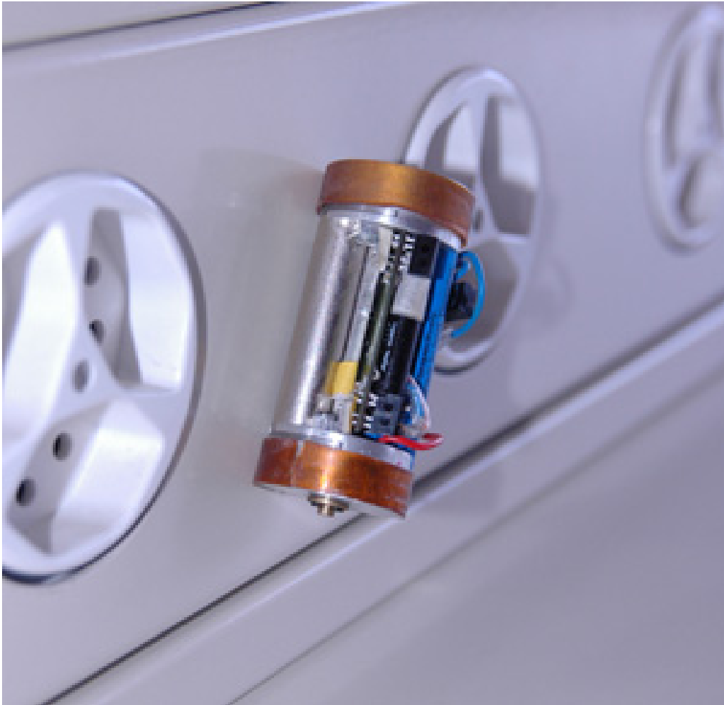
Figure 9: Cy-mag3D: Miniature climbing robot from Laboratoire de Systemes Robotiques (LSRO), Robots group, Ecole Polytechnique Federale de Lausanne (EPFL)
