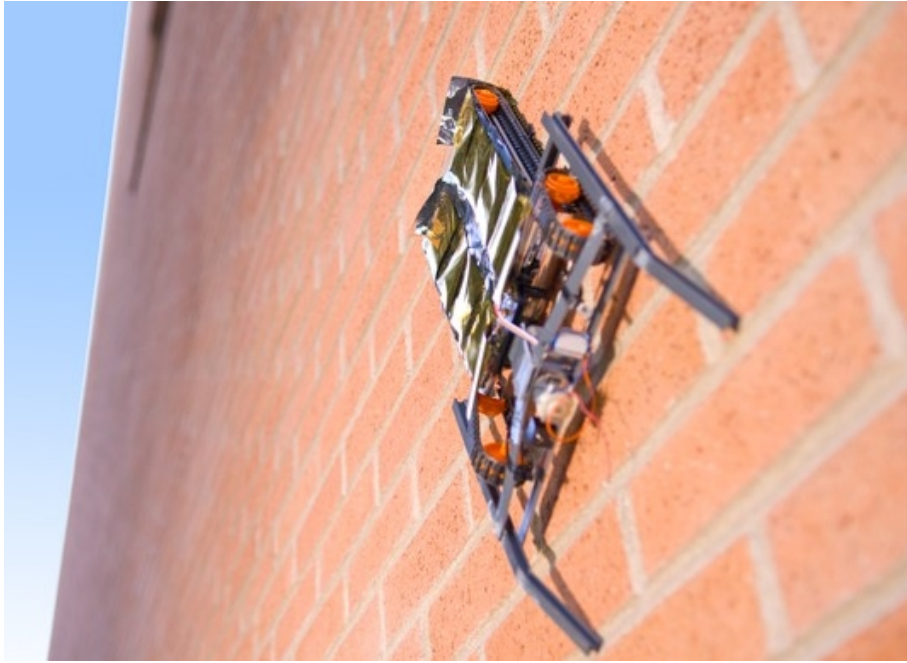
Figure 13: SRI International wall-climbing robot using a new electrical adhesive technology called compliant electroadhesion.
