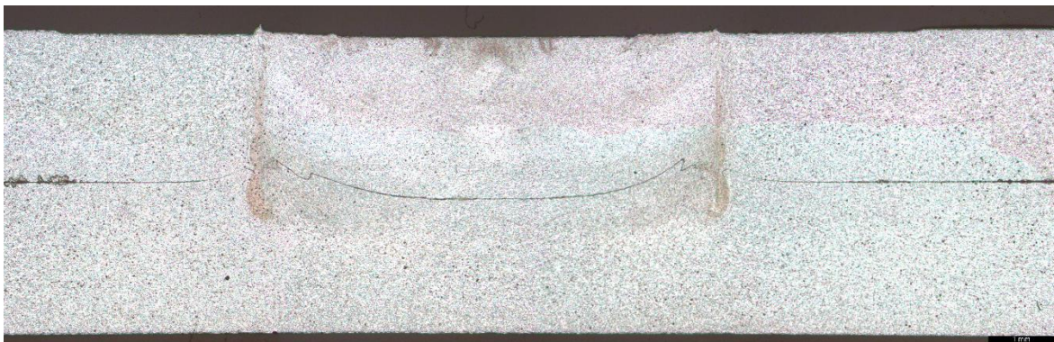
Figure 4.6 – Macrograph of the cross-section of condition O (FR=1.6; PD=3.6; RS=3000)
