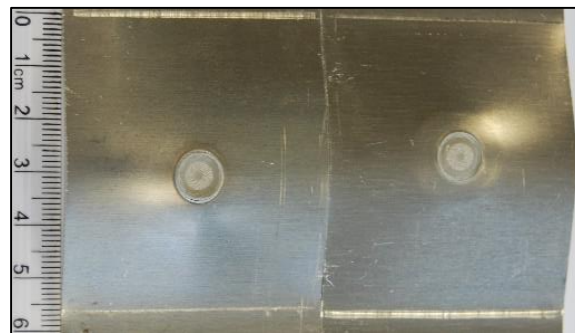
Figure 4.16 – Fracture mode for all CTS specimens
