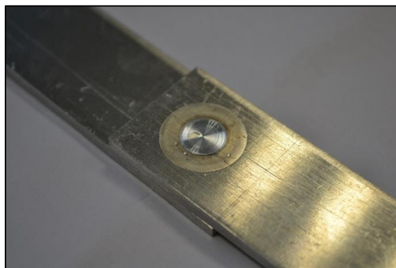
Figure 4.1 – Example of a Friction Spot Weld in AA5454-H22
