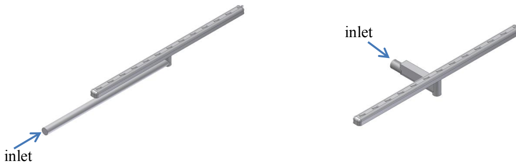
Figure 3-13: Illustration of the earlier designed air duct geometry (left) and the further version (right). The reason for the direction modification was to become an equal air distribution at the nozzles.
