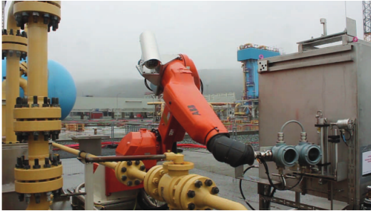
Figure 1.2: A robot locate in potentially explosive environment, among pipes carrying gas [1].
