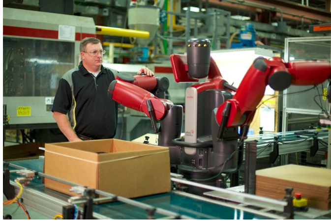
Figure 1.1: Baxter robot with coworker in a factory, collision avoidance is of vital importance to guarantee the safety of the coworker.
