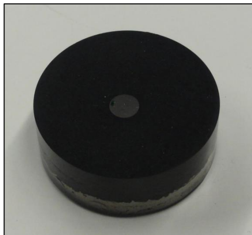
Figure 21 – Cross section into a resin body with 40 mm of diameter.
