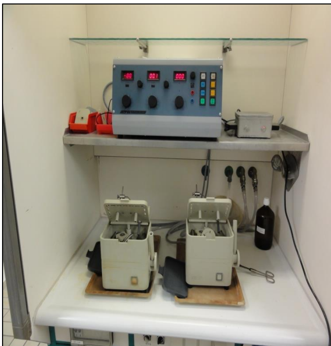
Figure 23 – Equipment used in electropolishing (University of Kassel).
