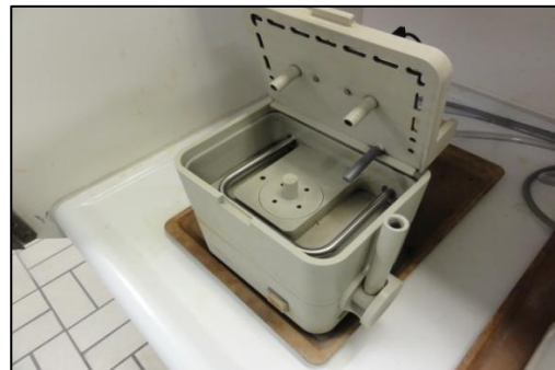
Figure 24 – Polishing unit used in electropolishing (University of Kassel).
