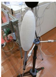
Figura C.5 - Indoor Comfort Analyser Type 1213 da Brüel and Kjær - Sensor de temperatura operativa
