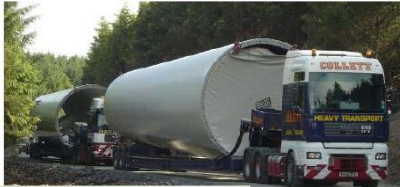
Figure 3. Transportation of steel tubular tower segments.
