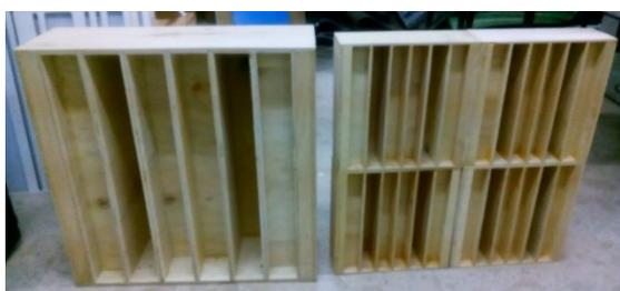
Figura 4.7 – Painel QRD\_60 (Esq.) e Painel QRD\_30\_4I (Dir.)
