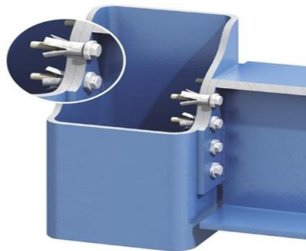
Figura 2.4 - Sistema "HolloBolt" (lindapter@, 2015)
