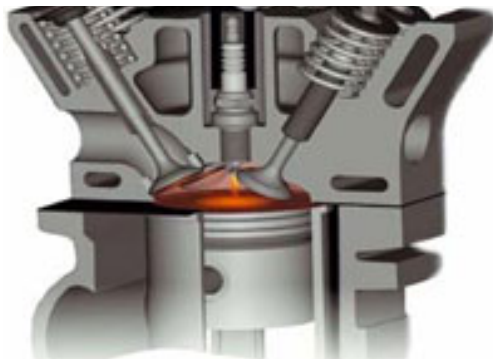
Figure 2.14. Schematic example of a combustion chamber with the piston at TDC [10].
