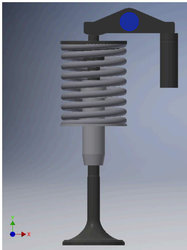
Figure 0.18. Valvematic's finger follower mechanism designed in Autodesk Inventor 2016.
