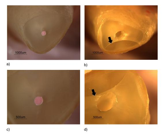
**Figure 2**: Photomicrographs of one tooth belonging to group 1, before (a, c) and after (b, d) root-end cavity preparation. No cracks are visible before, and one intradentine crack becomes evident after root-end cavity preparation (arrow in b and d).
