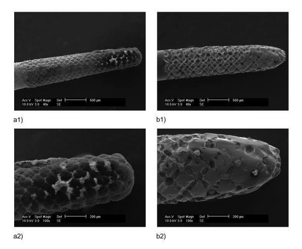
**Figure 2:** a1) / a2) – TOF-2 tip after use (40x and 100x magnification); b1) / b2) - Prototype tip after use (40x and 100x magnification).
