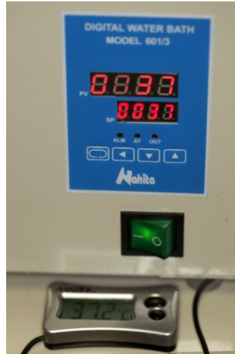
Figure 3: Double temperature monitoring of thermostatic bath with digital thermometer.
