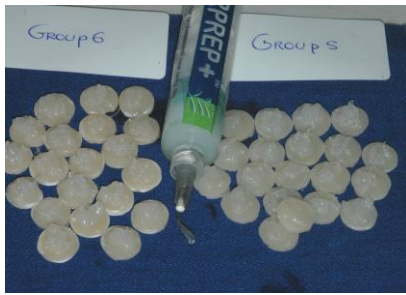
Figure 7. PowerPrep+™ was applied to the surface of specimens.
