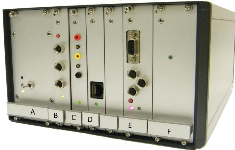
Figure 12 - Multichannel Platform. (A) Power Supply; (B) APW module; (C) ECG probe integrated with synchronization module; (D) PWV module; (E) PPG module; (F) NI6210
