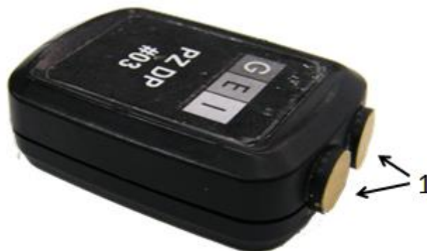
Figure 18 - Double headed probe. (1) Thin film PZ sensors.
