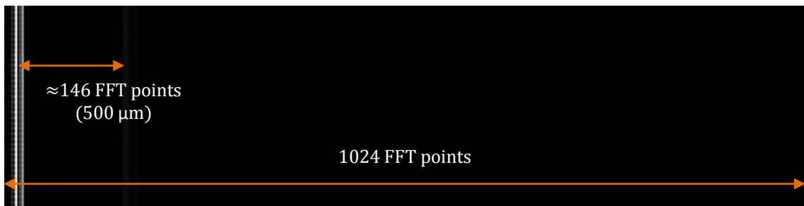
Fig. 79 - Image of the A-Scan for a sample mirror in position 0 and 500 \mu\text{m} . The galvo is not moving. The first A-Scan corresponds to the PSF of the system at z = \Delta z .
