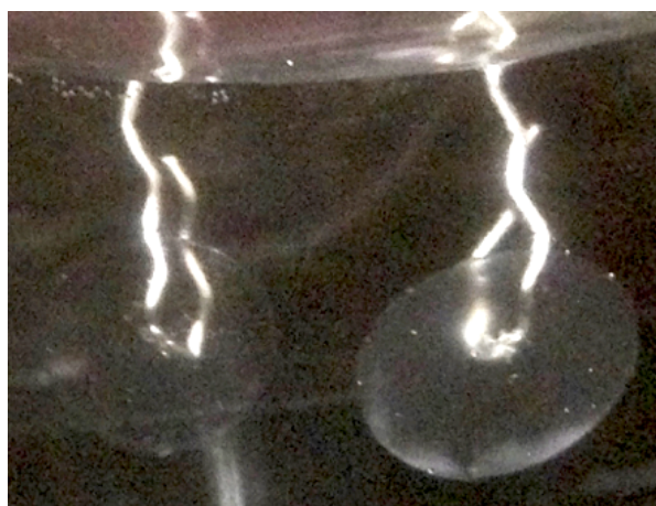
Figure 17 – SCLs with (on the right) and without (on the left) capsules while degassing.
