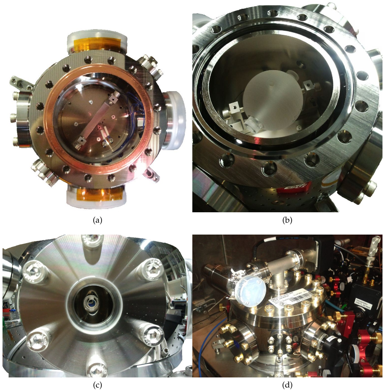
Figure 3.6: In (a) the thermistors at the base of the thermal shield and the fork-shaped support for the cavity can be seen. In (b) the spherical cavity is already assembled supported by two silver soft screws. In (c) it is possible to see the good optical access of the cavity through the windows. In (d) the cavity is already in vacuum with the tee flange connected to a corner valve and to the 2l ion pump.
