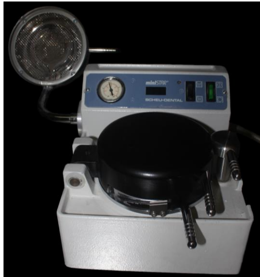
Figure 2: Thermal forming machine used to fabricate custom-made MG ( MiniSTAR , Scheu-Dental, Germany).
