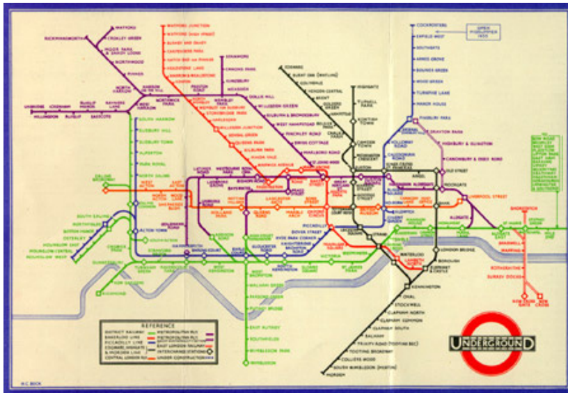
Fig. 20 Re-design of the London’s underground network, using schematic representation, by Henry Beck in 1931.
