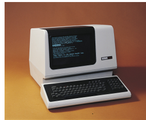
Figure 2.3: The VT100 video terminal used a command line interface.
