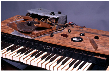
Figure 2.22: Touch-sensitive music synthesizer built by Hugh Le Caine.
