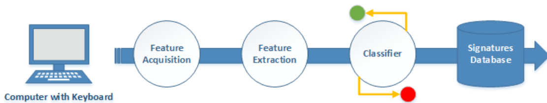
Figure 2 - A General Framework for the Keystroke Dynamics Evaluation Process
